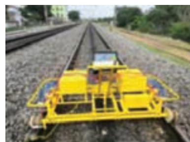
Digital Ultrasonic Double Rail Tester new technology B-Scan
