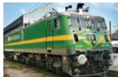
WAG 9 with IGBT based propulsion system
