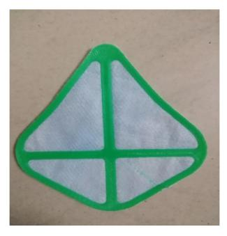
The filters of these reusable masks have also been developed using 3D printing. Further, Dr. Zambad says that the masks have been found to have bacterial filtration efficiency higher than 95%. "In this project, for the first time, we used 3D-printers to make multilayer cloth filters to precisely fit for plastic-moulded or 3D-printed mask covers".
