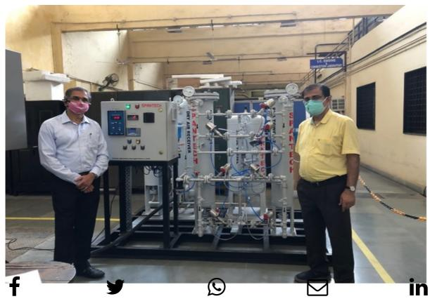
How can the nitrogen unit be converted into an oxygen unit? "It has been done by fine-tuning the existing Nitrogen Plant setup and changing the molecular sieves from Carbon to Zeolite" says Prof. Milind Atrey, Dean (R&D), IIT Bombay, who led the project.
