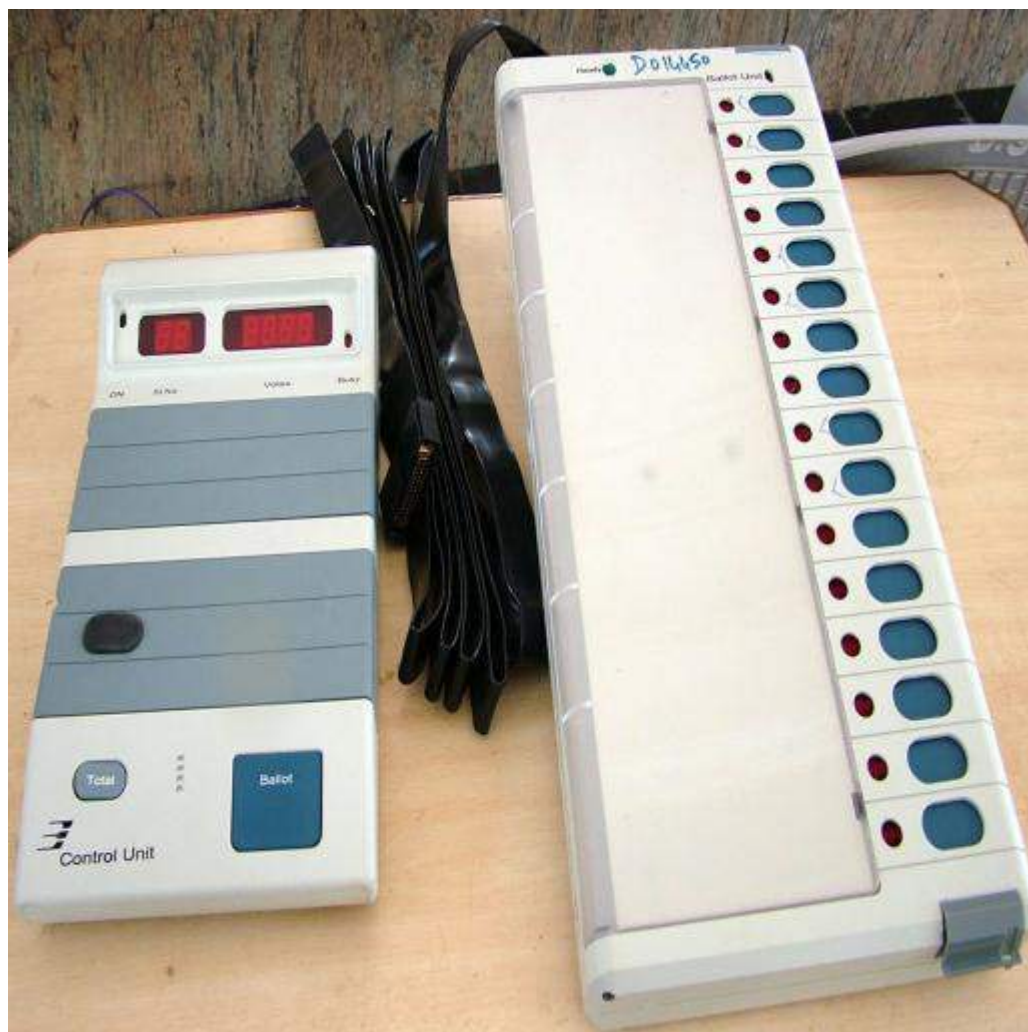
A Direct Recording EVM of the kind used in India consists of a Control Unit (left) and a Ballot Unit (right) connected by a cable. The Control Unit is operated by the election staff while the voters cast their ballot on the Ballot Unit.
